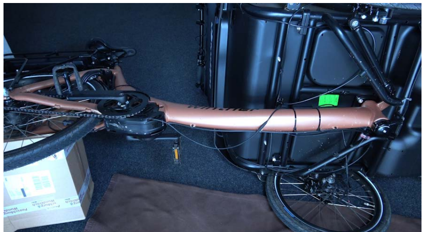
Fig. 13 Cable routing to the rear
