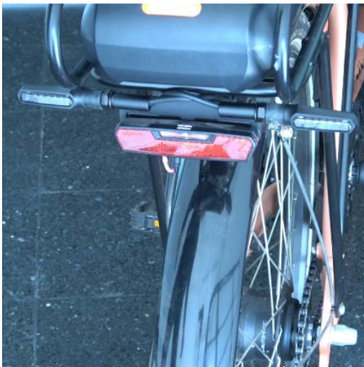
Fig. 12 Mounting position of blinker bracket on rear light
