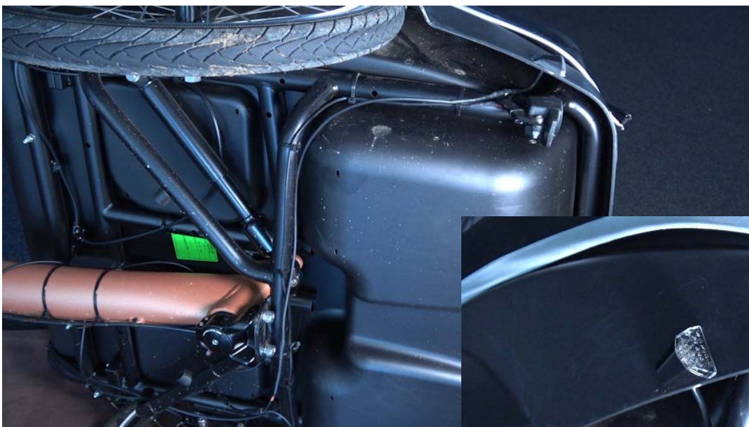
Fig. 9 Cable routing for the indicators
