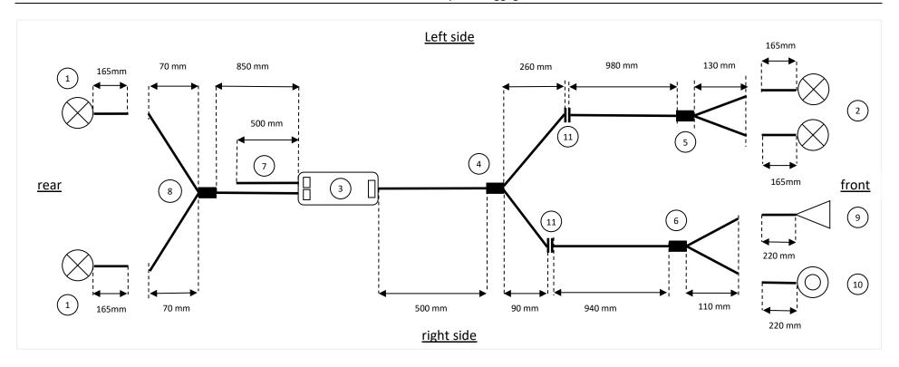
All lengths are subject to a manufacturing tolerance of +/- 10 mm. We reserve the right to make changes in the interests of technical progress. Splitter length 30mm +/- 10mm tolerance, 15mm per cable side +/- 5mm
